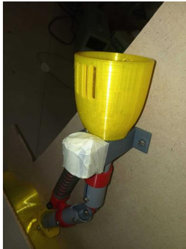
Fig. 2: Spring-integrated two-link canine prosthetic limb prototype.
