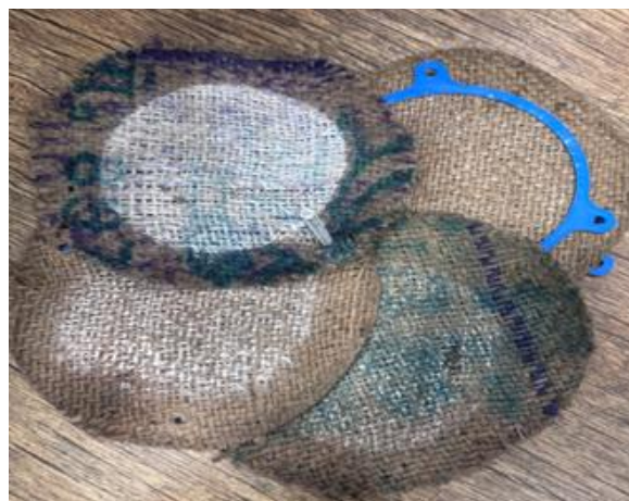
Figure 6: Particle deposition on fiber plates.
