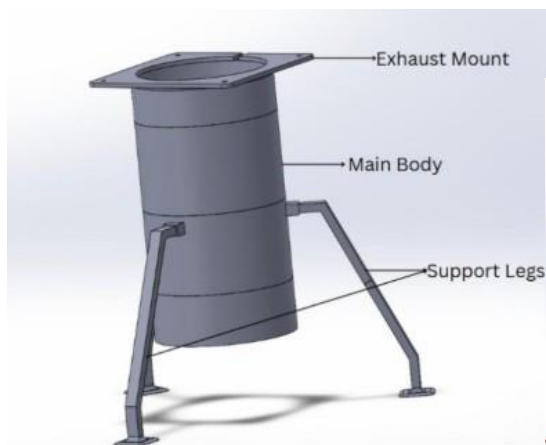
Figure 5: Diagram of filter (Orthographic view; SolidWorks)
