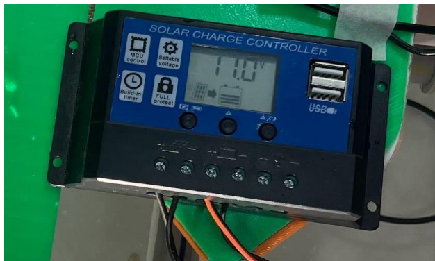
Fig4. MPPT Solar charge controller charging the battery
